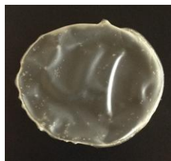
Fig. 1 Physical appearance of unplasticized corn husk cellulose laurate film
